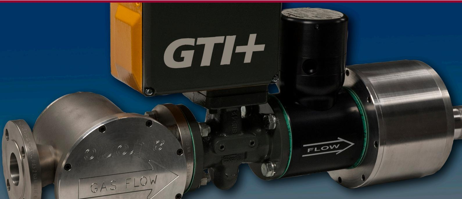
Since the AGV5 is rated to a higher pressure, the gas train can accept gas supply pressure of up to 50 psig, eliminating the need to reduce higher gas supply pressures to lower gas train inlet pressures with an added primary regulator.
